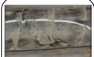
Hole in hose cover that exposes reinforcement
